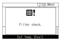
• If the air conditioners are operated while "**!!**" is displayed, then "Filter check." is displayed. Press an operation button while it is displayed or leave it for at least 5 seconds and the display will disappear.
