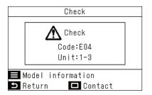
When an error occurs in the air conditioner, the check code and the indoor unit number flash on the display of the remote controller.
