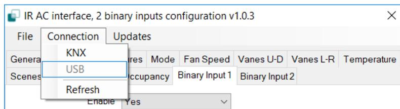
**USB connection is faster than KNX connection.** Notice that USB is only available for the IR parameters download (see [5.1 General configuration](#)).
