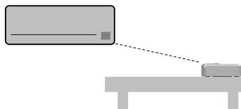
Figure 3.2 IR emitters and IR receiver location
