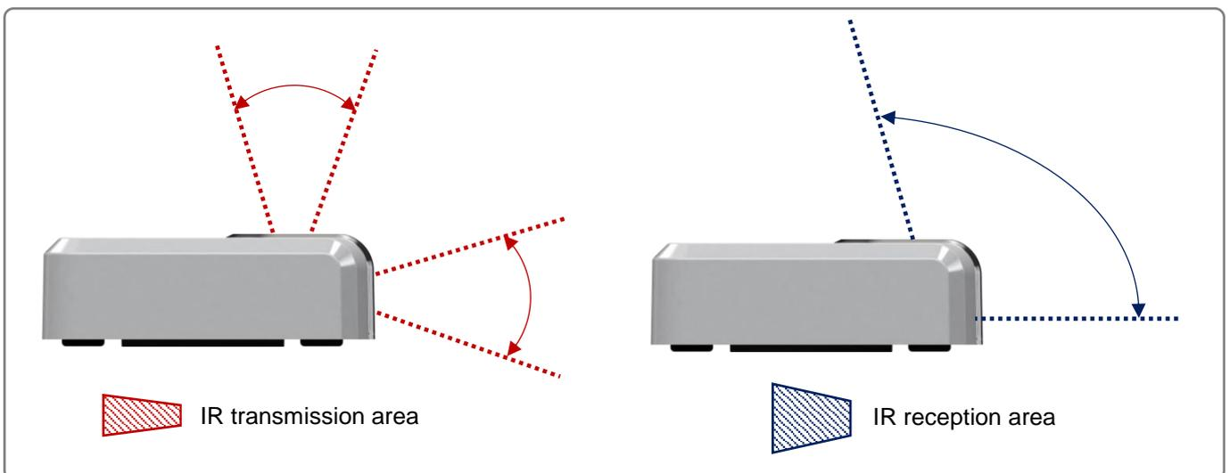
Figure 3.1 IR emitters and IR receiver location
