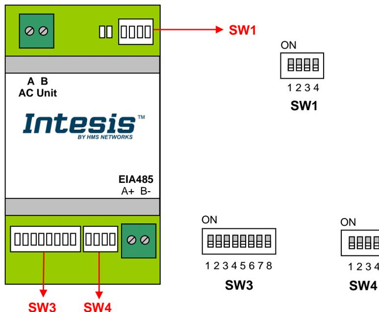
The following tables apply to the interface's configuration through DIP-switches:
